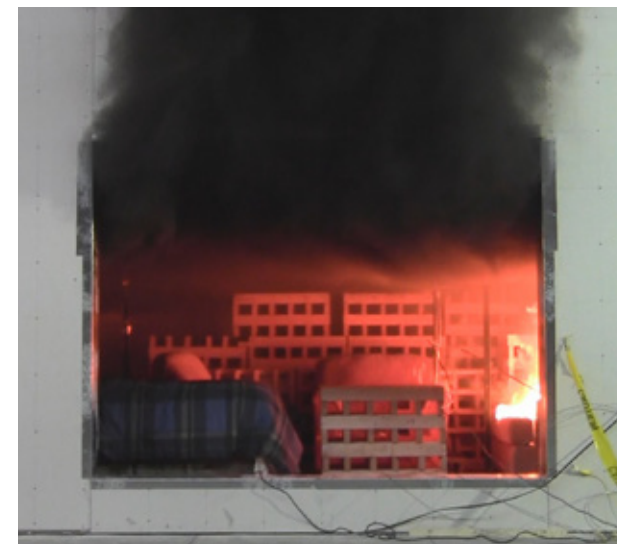
Allumage de la charge combustible © Photo: Nordic Structures
