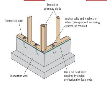
StrandGuard® TimberStrand® LSL framing materials are intended for use in aboveground, protected applications such as sill plates and studs. The American Wood Protection Association (AWPA) standards classify such applications as Use Category 2.
