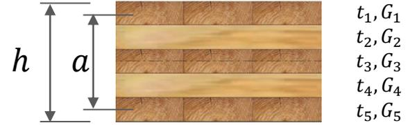
$$s = \frac{a^2}{\frac{t_1}{2} \frac{1}{G_1} + \sum_{i=2}^4 \frac{t_i}{G_i} + \frac{t_5}{2} \frac{1}{G_5}}$$
