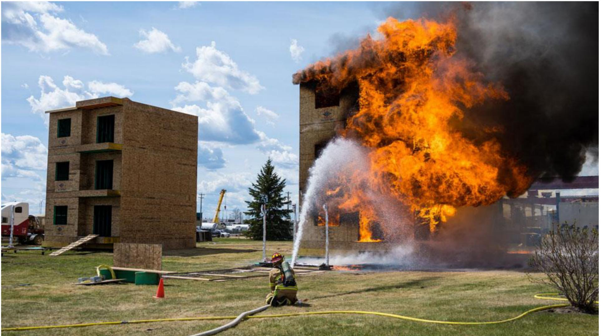
**BARRIERTEK** — BarrierTek conducts a large-scale test of fire suppression technology. The Alberta company built two identical structures and then treated one with its fire-prevention coating designed to protect structures during construction.
